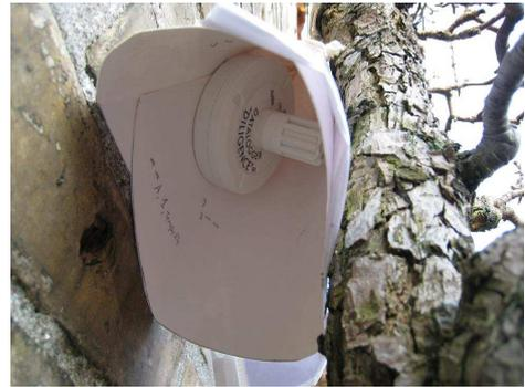
**Figure 5.** Climate logger positioned in Alnarp seen from below and enfolded by paper cap as protection.
