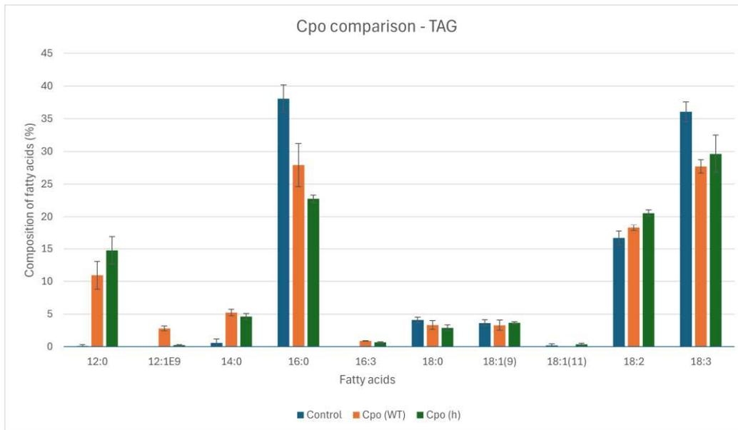
Figure 17. Comparison of fatty acid composition (%) in TAG in *Nicotiana benthamiana* leaves infiltrated with treatments control, *Cpo* (WT) and *Cpo* (h).  $n = 3$  biological replicates. Error bars represent standard deviation.
