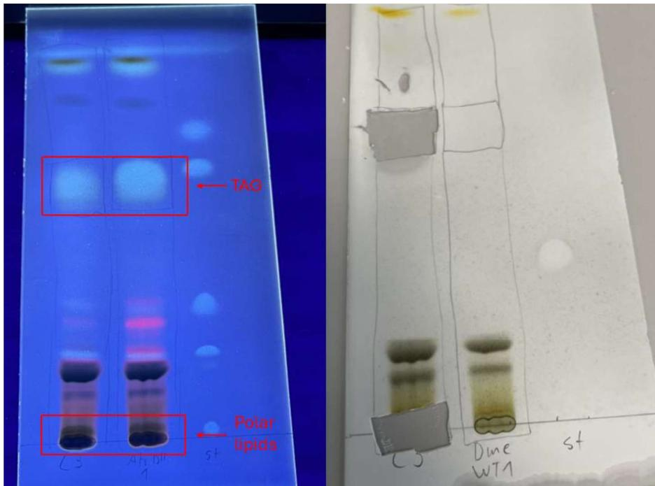
Figure 14. Lipid separation with thin layer chromatography (TLC). On the left is a TLC plate view under UV-light with areas with TAG and polar lipids are marked in red. The right image illustrate areas of TAG and polar lipids scraped off and included in the lipid analysis.
