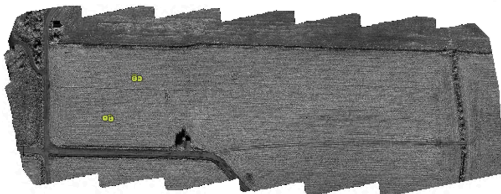
Figure 7. NIR reflectance raster overlaid with polygon boundaries in QGIS for zonal statistical analysis.
