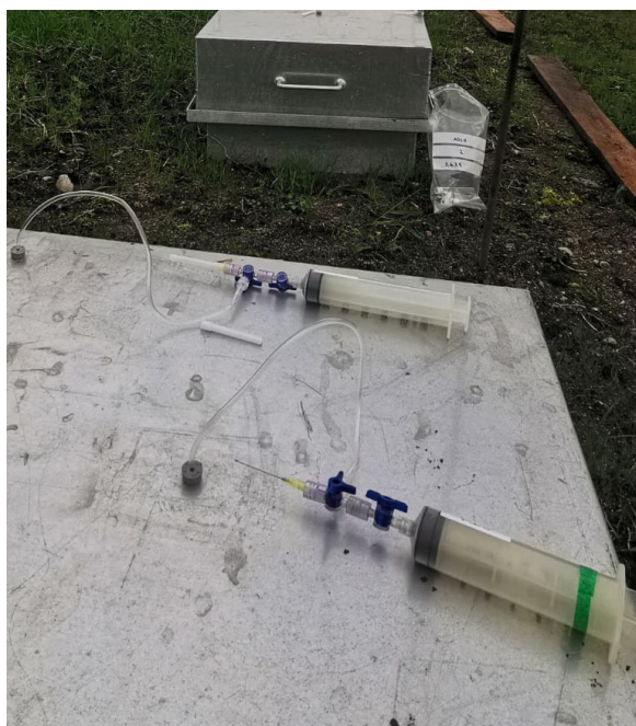
Figure 5: Manual sampling with syringes and vials for later analysis with gas chromatography. Photo: Johanna Maria Zimmermann
