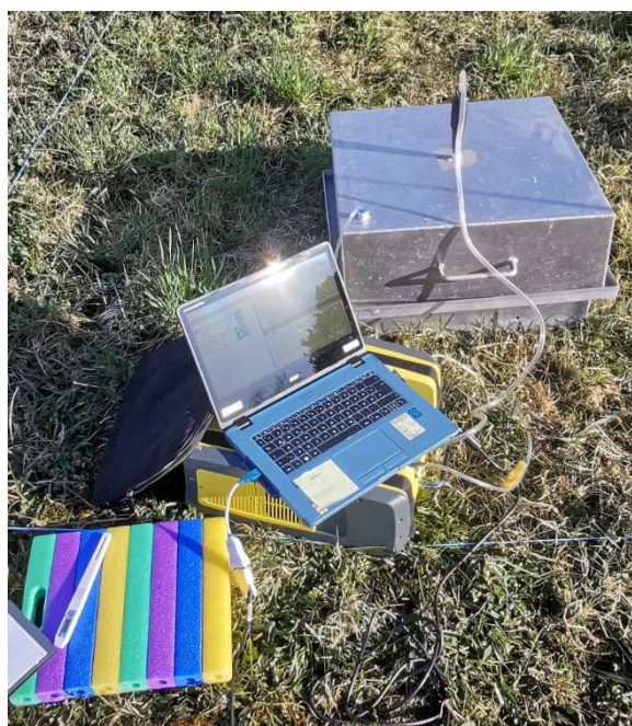
Figure 4: Gas measurements using GasMet FTIR analyzer. Photo: Johanna Maria Zimmermann
