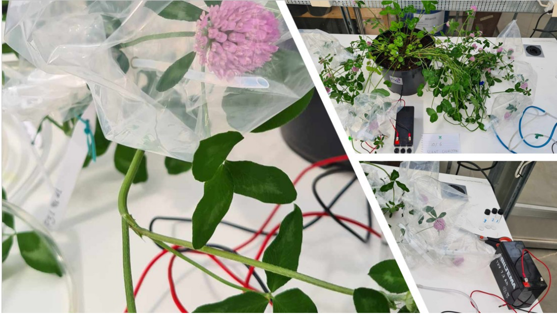
Figure 4. The setup of floral VOC collection inside a greenhouse chamber at SLU
