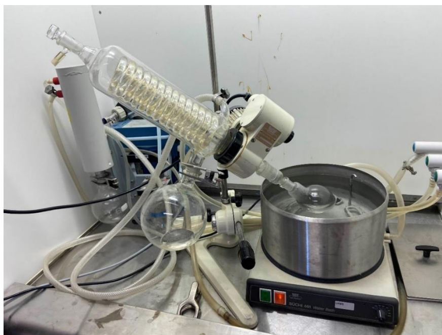
Figure 2-8 Rotary Evaporator system for HPLC isoeugenol extraction
