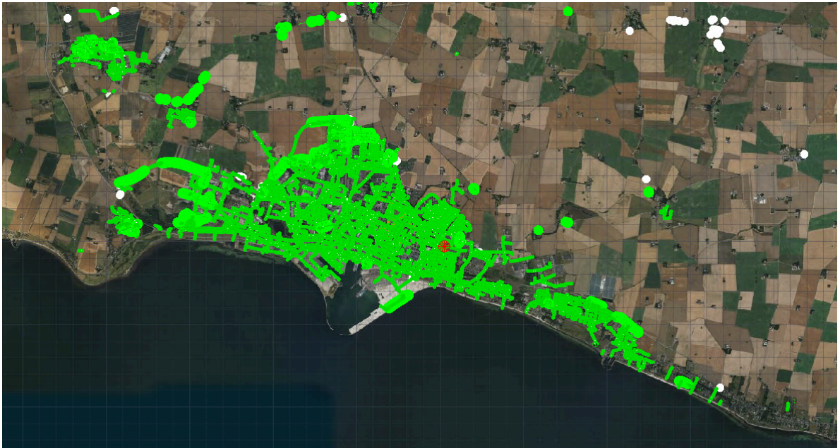
Figure 34: Drainage system network in Trelleborg.
