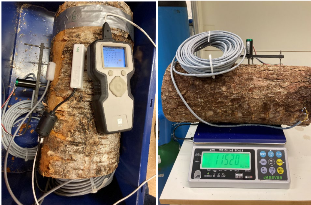
Figure 3. Log equipped with point dendrometer, heat pulse sap flow sensor, TEROS water content sensor, and TEMPOS thermal properties sensor (left). Log weighed on scale with point dendrometer attached for measuring gravimetric water loss (right).
