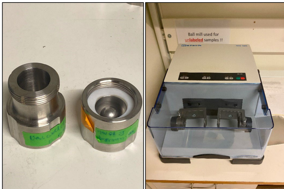
Figure 3. Pictured on the left is the 10ml hollow shells with the stainless steel ball. The ball mill grinder that was used is pictured on the right.
