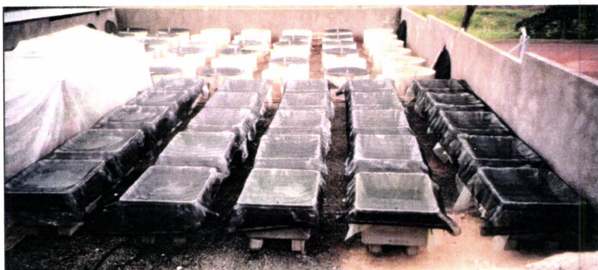
Figure 4. All mesocosms covered with sunshade (40 % reduction of insolation).
