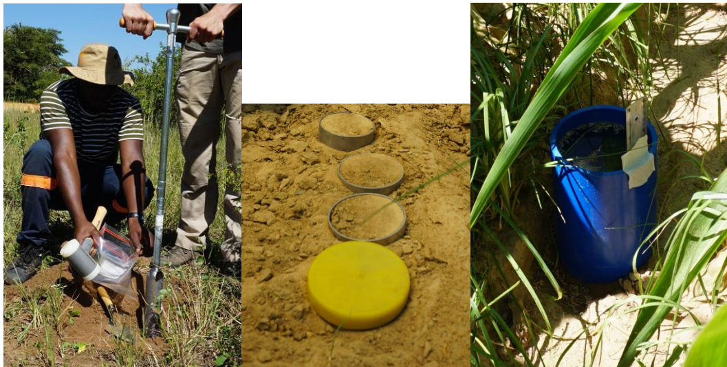
Figure 3: Images of some sampling process in the field. Left: loose soil sampling with an auger for chemical analysis, centre: soil cylinders halfway inserted for bulk density, right: infiltration rate measurement with an inserted infiltration tube, a fixed rule.
