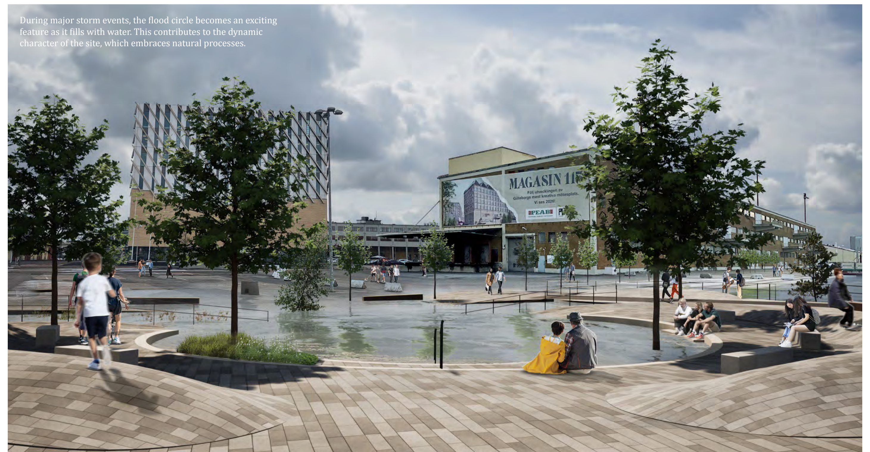
Sea level rise of a 50-year storm event in 2070: +2.00 At a storm event of this level, sea levels will rise and fill the Green-Blue Spine and the first level of The Flood Circle temporarily. The lowest lying blast rock planting will also get filled by its overflow connection to the mineral edge.
