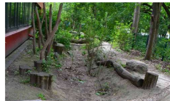
Fig. 38. Natural obstacle course-like lane that functions as a bioswale as well.
