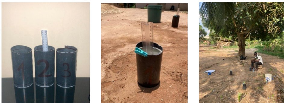
Figure 13. PVC ring infiltrometers performing infiltration methods in the field
