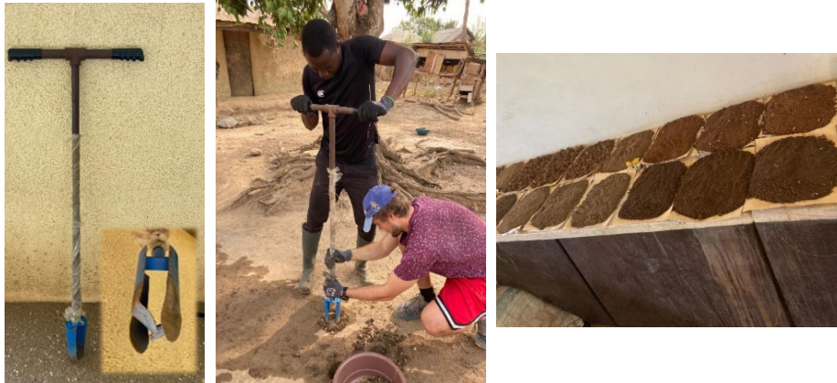
Figure 12. From left to right: Soil auger, taking of composite samples and drying of composite samples
