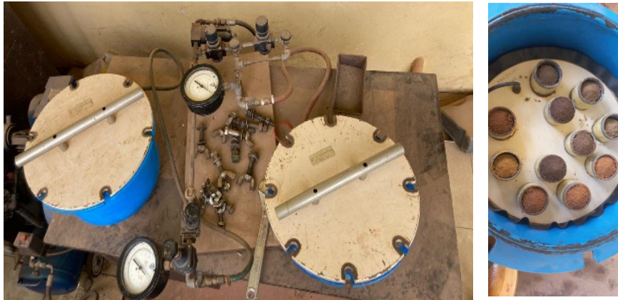
Figure A 1. Pressure plate analysis of loose, disturbed soil samples to retrieve FC and WP
