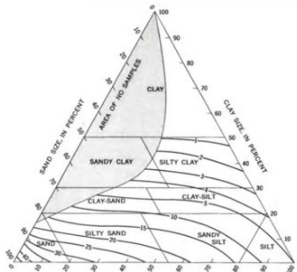
Figure 16. S_y according to USDA soil texture triangle as in Richey et al., 2015
