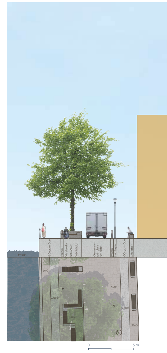
Section of Östra Ågatan and Västra Ågatan. By converting the street into a pedestrian area with one-way traffic, the streets can offer more space for walking on either side of the street. They can also accommodate zones for stay, in a variety of spatial sizes, both smaller spaces with vegetation under the tree crowns and in larger spaces without vegetation between the groups of trees.
