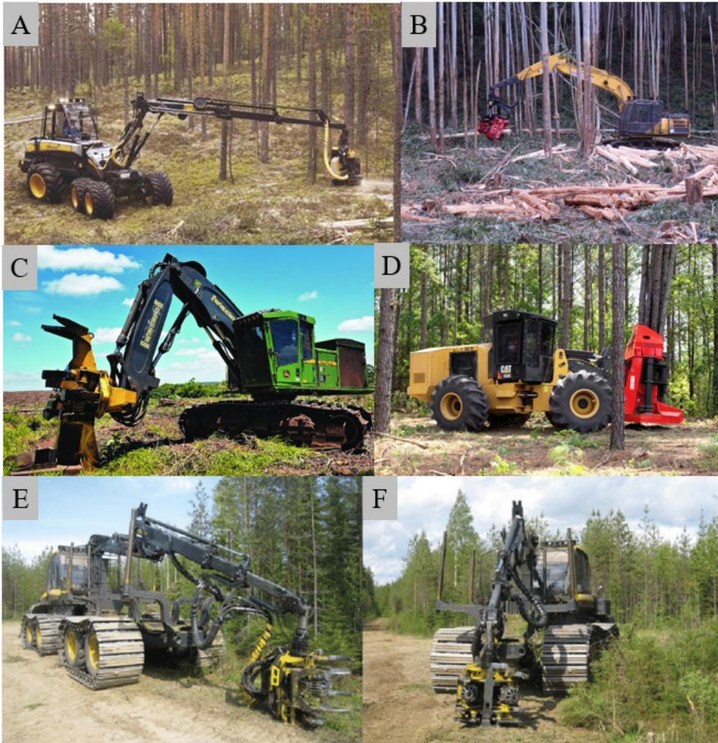
Figure 1. Various types of machines utilized in timber harvesting, A: purpose-built harvester (Billingsley et al. 2008), B: excavator-based harvester (Mcewan et al. 2016), C: purpose-built swing-boom feller-buncher (Rocha et al. 2022), D: purpose-built drive-to-tree feller-buncher (Anon 2023a), E and F: purpose-built harwarder (Laitila & Väätäinen 2020)
