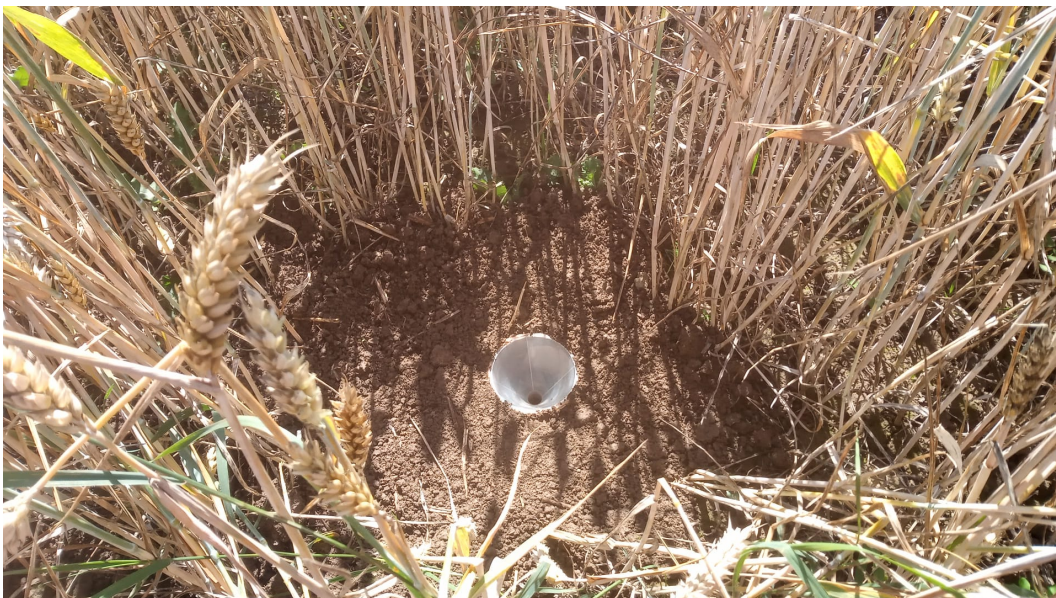
Figure 4. Time-turning traps buried in the soil were used to trap carabids in two-hour intervals to allow interval-based collection and to further determine species-specific climate niches. It consists of a box with a funnel that is dug into the soil with the opening of the funnel in line with the soil surface. Within the box, there is a rotating wheel equipped with vials filled with water and dishwashing liquid. As the carabids fall through the funnel they are caught in the vials, with one vial representing a two-hour interval. Photo: Cassandra Vogel
