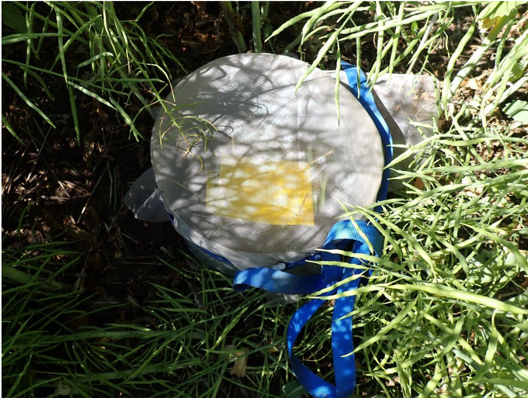
Figure 8. Emergence trap. Photo: Plant Protection Centres of the Swedish Board of Agriculture.
