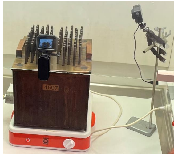
Figure 5 Mattsson cooker during cooking with timelapse recorded by GoPro cameras.
