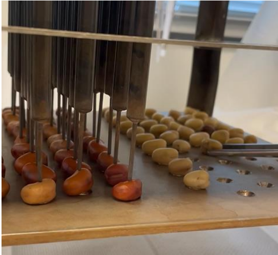
Figure 4 Placement of seeds under plungers in the seed rack of Mattsson Cooker.
