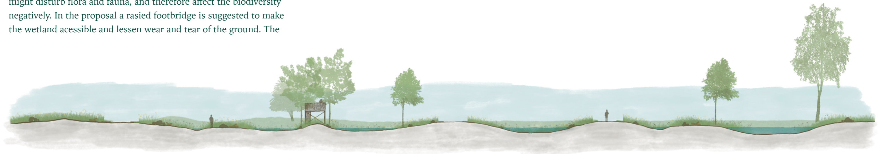
Section of the wetland with the forebay to the right and meandering wetland to the left.
