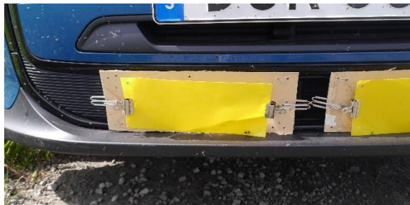
Figure 3. Sticky traps mounted on a car. The sticky traps (yellow) are mounted to a hard cardboard plate (brown) with metal clippers. The cardboard is mounted to the air intake of the vehicle with wire.
