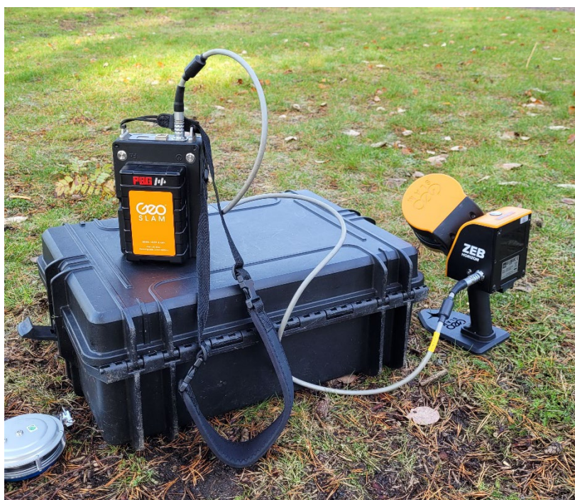
Figure 2. GeoSLAM ZEB Horizons scanning head with a handle and a data logger.
