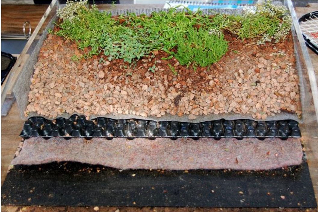
Figur 1. Construction sample of a green roof system (thingermejig 2006) ( CC BY-SA 2.0 ).
