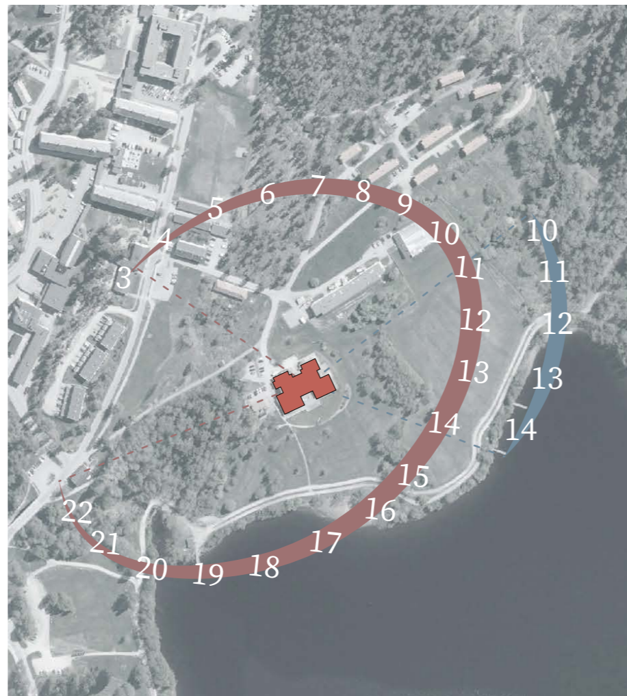
Figure 18 A diagram of the sun's location according to the season: Reds are the longest day. Blue is the shortest day.
