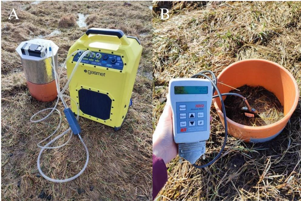
Figure 5. (A) Gas emission measurement with Gaset and (B) soil temperature with WET sensor. (Photos: Fanny Otterlin Karlsson).
