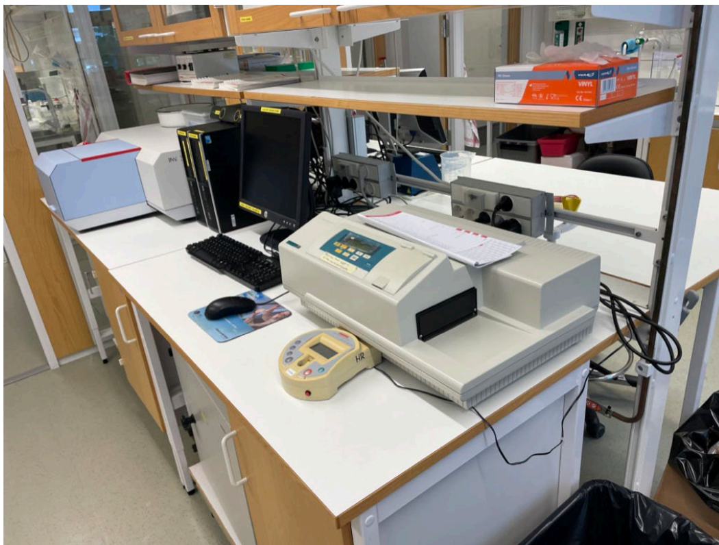
Figure 4. SpectraMax® Plus 384 Absorbance Microplate Reader used for analysis of Mn peroxidase activity in the foreground. LS50B Luminescence Spectrometer used for analysis of peptidase activity in the background.
