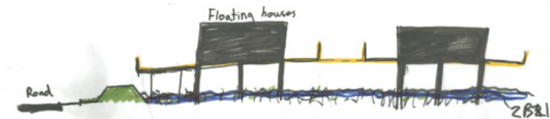
Section 2B1-2B1 shows the elevated buildings with a deck between them, the section is not in scale.
