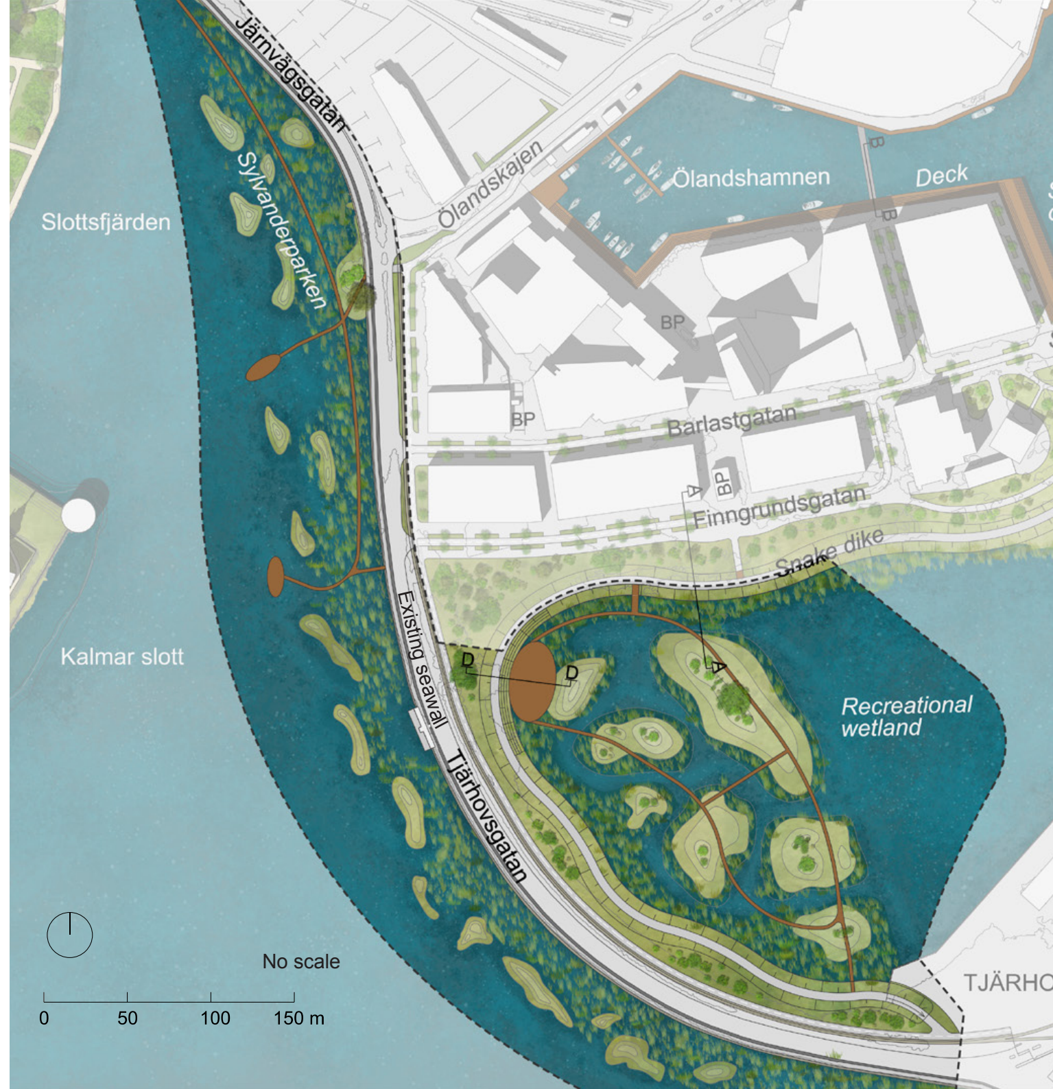
Fig. 125. The recreational wetland has islands formed using the landfill material from the place where channels were made by excavating the landfill. The wetland and the barrier islands in Sylvanderparken and along the road were created to be used as buffers for storms (data from Lantmäteriet 2021 and 2022; Samhällsbyggnads-kontoret Kalmar kommun 2023).
