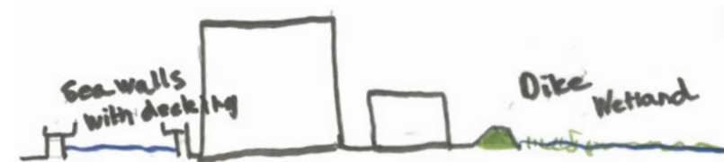
Section A1-A1 shows the area with various techniques, such as seawalls, dikes and wetlands. The section is not in scale.
