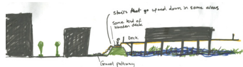
Section 2B2-2B2 shows how the dike could be used to access the elevated buildings, the section is not in scale.
