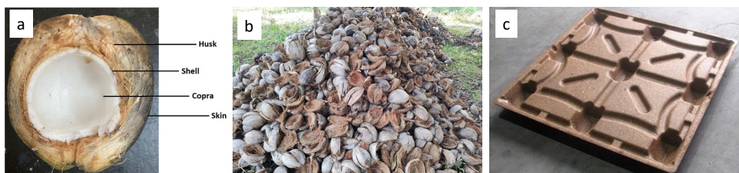
Figure 15 Exterior parts of coconut (a, 114), discarded waste coconut husks (b, 114), and binderless coir pallet (c, 114). Coir is the fibrous material obtained from the husk after processing.
