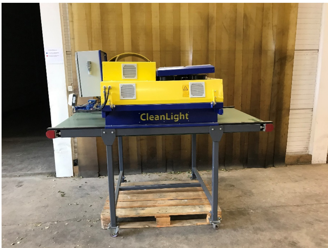
Figure 3 CleanLight machine used to carry out UVC treatments.
