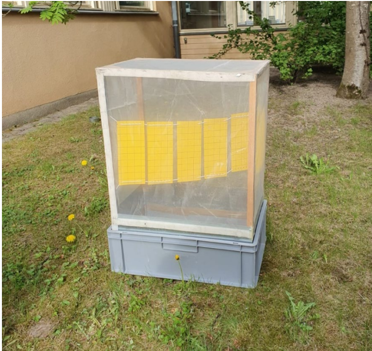
Figure 3. The mesh mesocosms, used for flight-experiments. I marked 6 species of insects with red, blue, or yellow fluorescent dust and released them together with unmarked control groups for all species. I hung five yellow sticky traps across the mesocosm to catch insects capable of flying. By this method, I could conclude whether the fluorescent dusts hampered their capability of flight. If more insects from the control groups were caught in the sticky traps compared to marked individuals, this would suggest that the dusts do hamper their flight capability.
