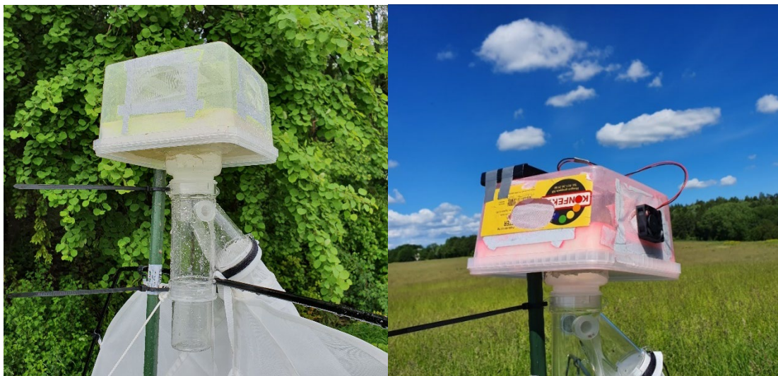
Figure 5 The novel trapping device in field. In the left picture, the trap has been painted with yellow dust and carries no fan. Notice the upside-down Malaise bottles glued to the lids of the boxes, attached to the Malaise traps. In the picture to the right, the inside has been painted with red fluorescent dust and a battery-driven fan is attached to one of the mesh-covered air holes.
