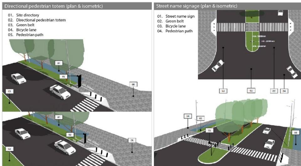
Figure 29. Crosswalk, directional pedestrian totem, and street name signage concept
