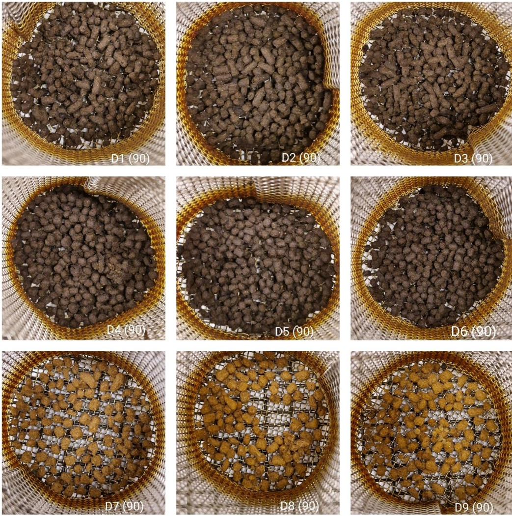
Figure 16. Pictures of experimental diets from water stability test 90min, dry samples. Control diet: D1-D3; BSF diet: D4-D6; Tonse diet: D7-D9.
