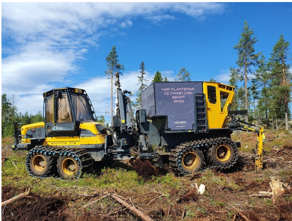
Figur 1. Plantma X planteringsmaskin (Foto: Sara Nilsson, Holmen Skog). Figure 1. Plantma X planting machine (Photo: Sara Nilsson, Holmen Skog).
