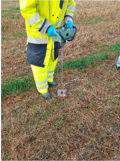
Figure 4. The penetrometer was pushed down vertically in the soil.
