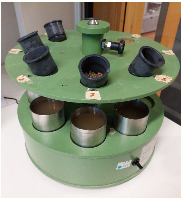
Figure 2. The picture shows the wet sieving apparatus with the containers containing soil above the metal containers containing rainwater.
