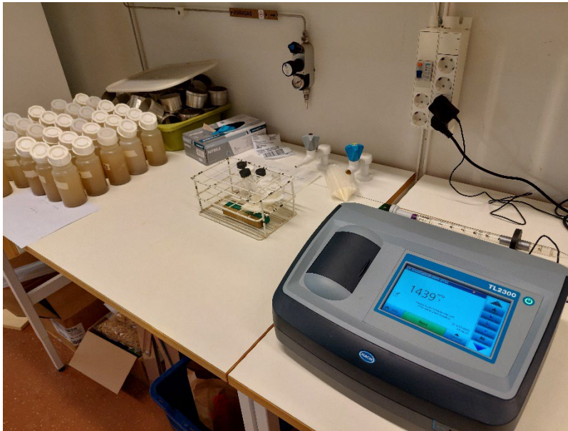
Figure 3. A picture of the turbidimeter, where the glass cylinder was placed below the black lid on the turbidimeter. The samples were in the bottles to the left.
