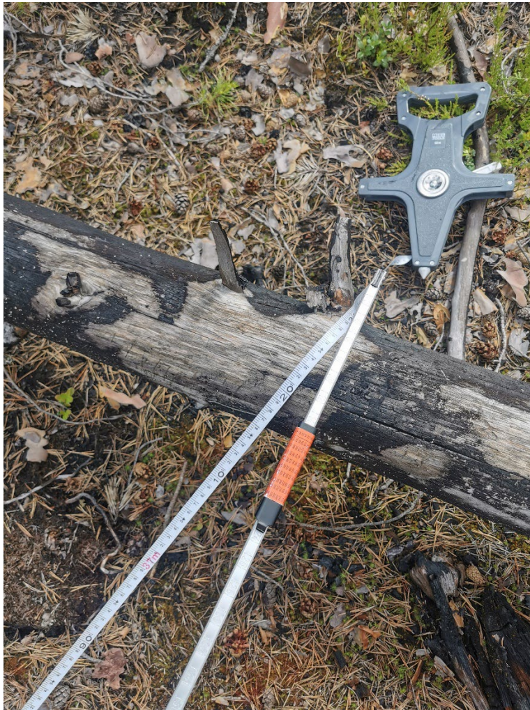
Figure 8. Diameter measuring of a downed pine in one of the transects in the wildfire site Gommorsberget. The consistent charring of the log indicates that this pine was downed and dead before the fire event.
