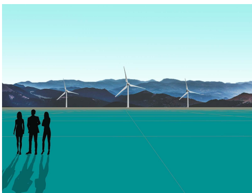
Figure no.24 The sight of the turbines at a distance of 1000 meters with good weather conditions and flat ground.
