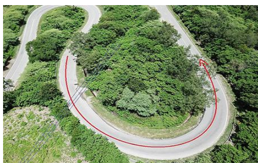
Figure no.19 Cornering is one of the most difficult issues during the transportation of turbine parts which requires prior study.
