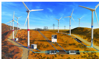
Figure no.33 Connecting the turbines to the substations and from there to the national grid through underground cables.
