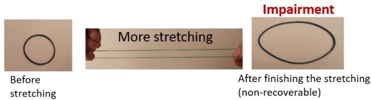
Figure 7: A schematic representation of the strength using an elastic material. The original form of the material is non-recoverable after the stretching applied on it.
