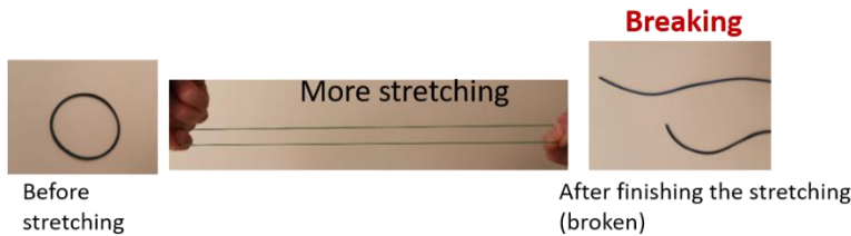
Figure 8: A schematic representation of the toughness modulus using an elastic material. The original form of the material is broken after the stretching applied on it.
