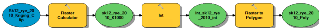
Figure 16. ArcMap model using a succession of tools to transform a raster layer into a vector layer. Blue box corresponds to model input, yellow boxes to tools and green boxes to outputs, produced in ArcMap.
