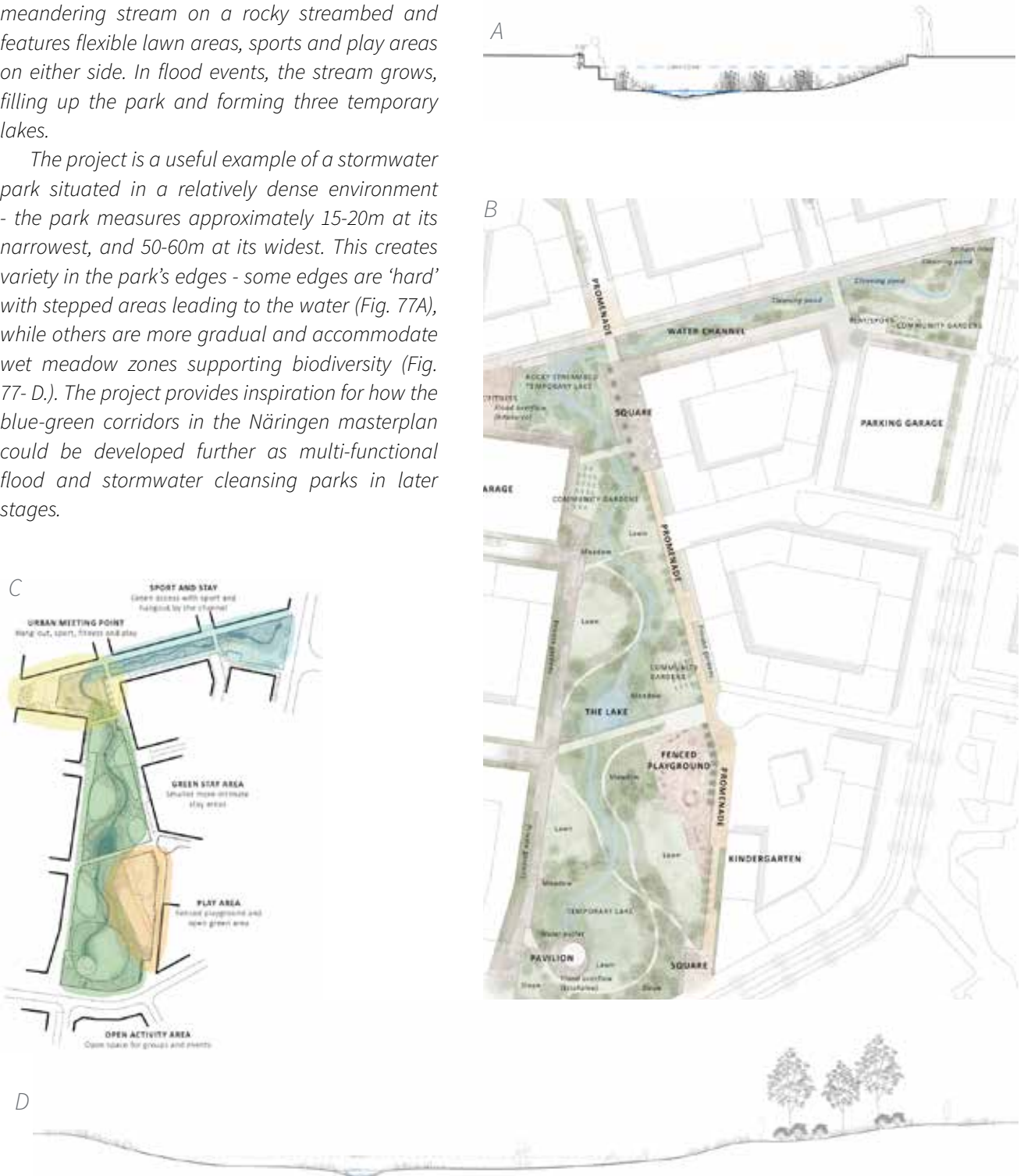
Figure 77: (ALL) Pihlajaniemi Stormwater Park design. A: Section of water channel. B: Plan. C: Activities Diagram. D: Section of stream and wet meadow. Source: Masu Planning
