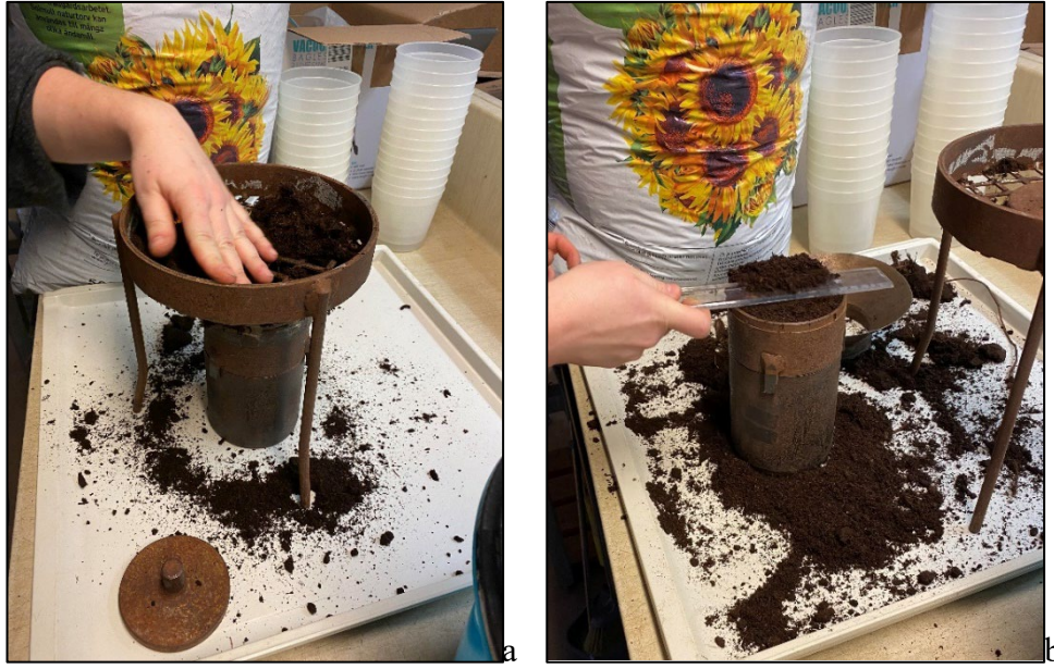
Figure 3. Bulk density measurements: filling (a) and excess removal (b) from iron cylinder.
