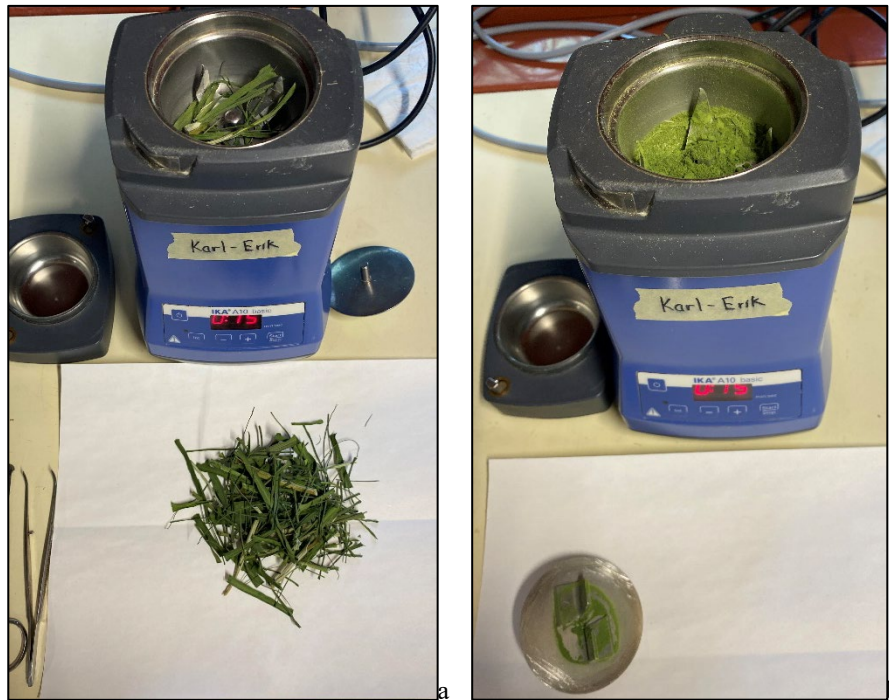
Figure 4: Dried (a) and milled (b) A. porrum biomass by IKA® A10 basic.
