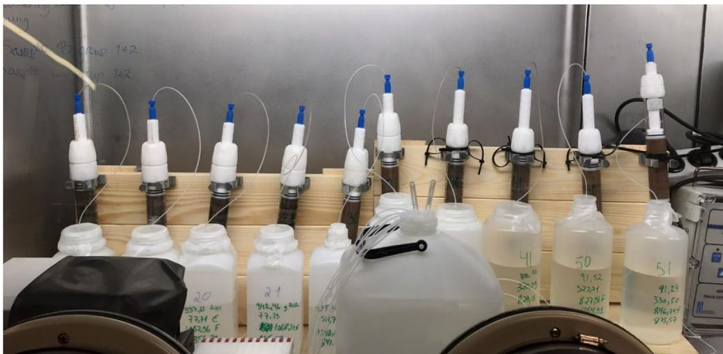
Figure 8. Long-term experiment columns with their respective eluate containers inside the glove box. Shown in the foreground is the collective AGW container. Photo taken by the author.
