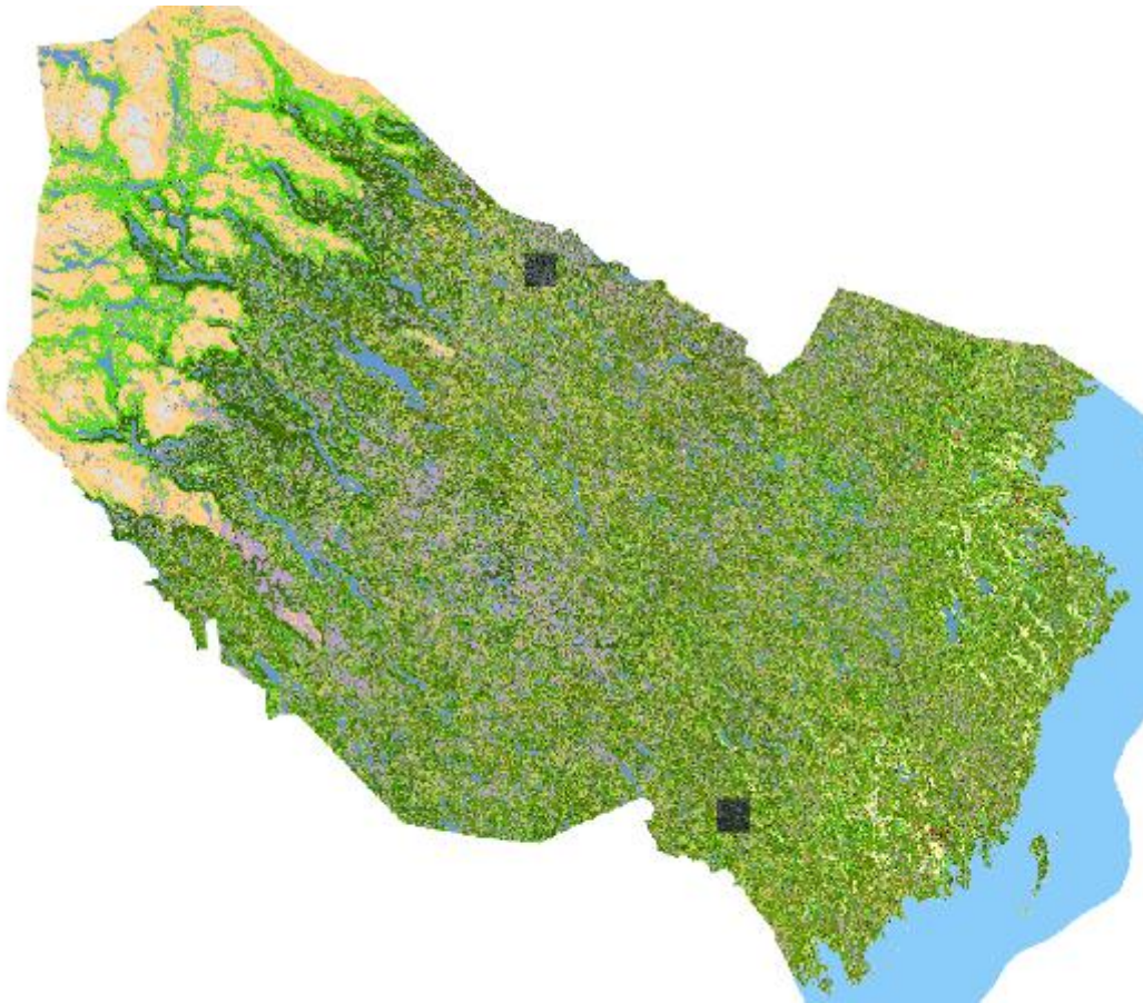
Fig 2. The QGIS canvas with the selected areas of study in Västerbotten. The darker squares are the 10 000 ha large study areas, consisting of 4 orthophotos each. The top left area is the inland area (coordinates: 726_63_00, 726_63_05, 726_63_50 and 726_63_55) and the bottom right area is the near coastal area (coordinates: 709_69_00, 709_69_05, 709_69_50 and 709_69_55), based on OrtoRgb050 epsg3006, © The National Land Survey. Background picture: “The National Land Cover” data layer for Västerbotten county in Sweden, 10x10m, © Swedish Environmental Protection Agency (2018).
