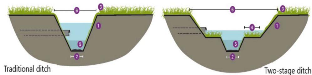
Figure 1. Cross section of a traditional trapezoidal (TD) ditch to the left and a Two-stage ditch (SD) to the right. 1, Side banks 2, bottom bed 3, bank top 4, terraces 5, base flow 6, high flow (Jordbruksverket 2016).
