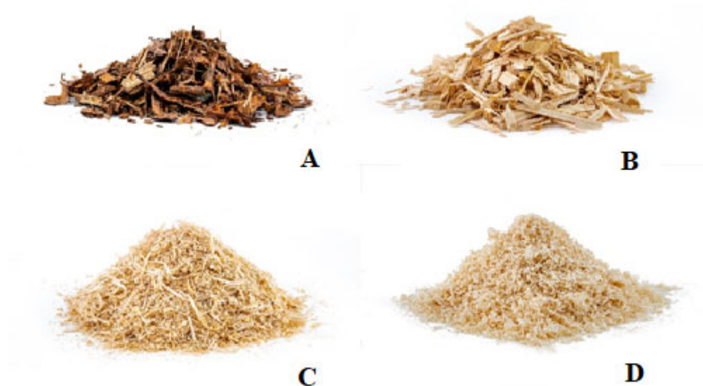
Figure 2. Picture of assortments, A = Bark, B = Cellulose-Chips, C = Sawdust and D = Shavings (Grabbe 2020).
