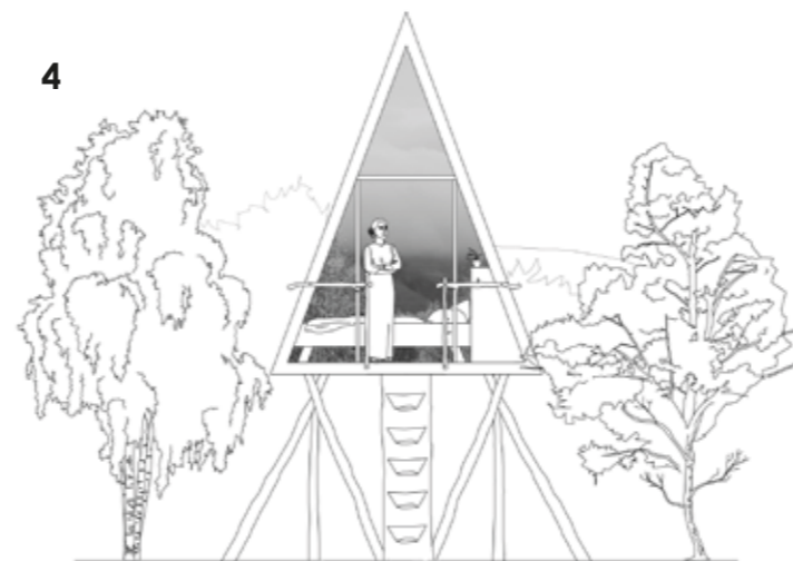
Figure 11. New accommodation for the tourist centre. The design is influenced by vernacular architecture. Material for details are gathered in the surrounding landscape. Glass gables create an immersive experience amongst the birch crowns, and the elevated structure provides privacy.
