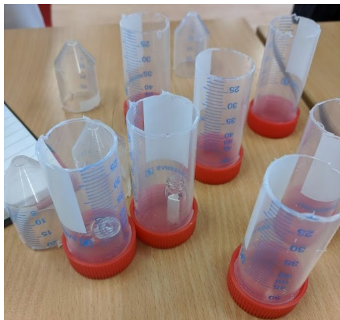
Figure 5. A 50 ml Falcon tube cut in half, with the open, cut-off end pointing upwards towards the dog. (Photo by Matilda Apelqvist)
