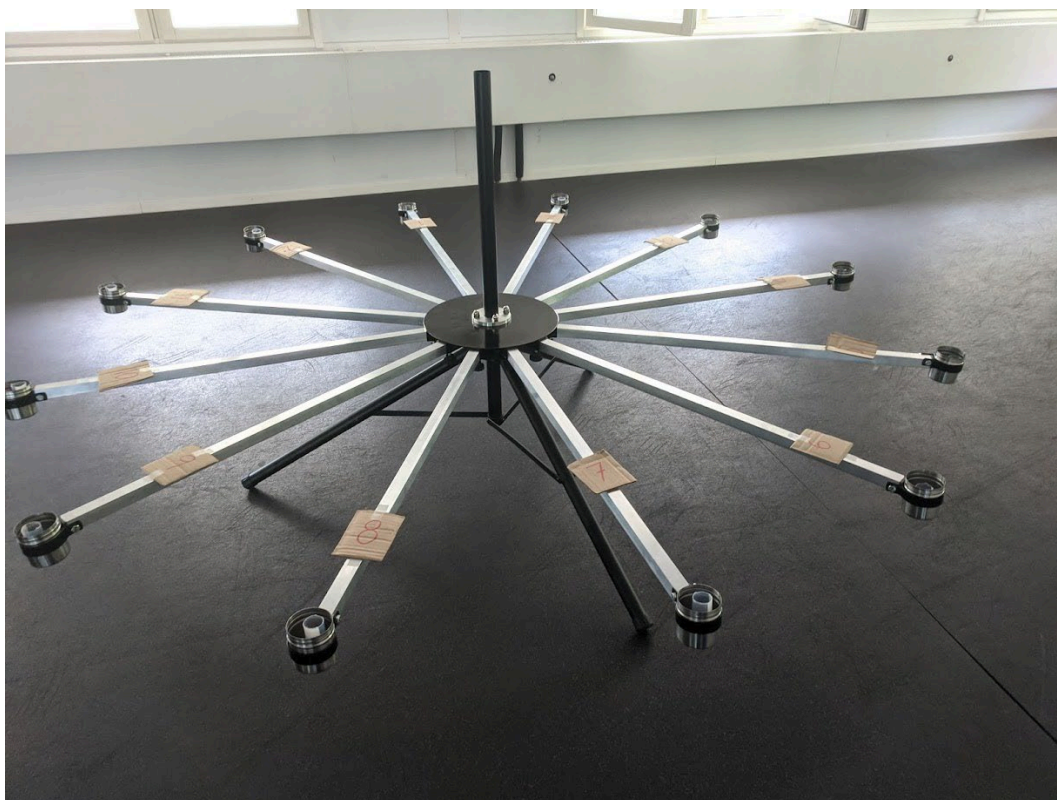
Figure 4. The scent wheel had a fixed centre and twelve arms reaching out from the middle. At the end of each arm there was a container in which the scent was placed. A 50 ml Falcon tube cut in half, with the open, cut-off end pointing upwards towards the dog, was placed in each of the containers of the arms of the scent wheel. (Photo by Matilda Apelqvist)
