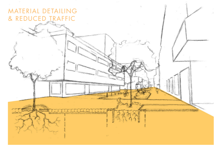
Figure 45. Material detailing in the ground cover can be used to pedestrianize the streets giving bikers and pedestrians priority to use the street. Adding softscape contributes to permeable surfaces along the street.
