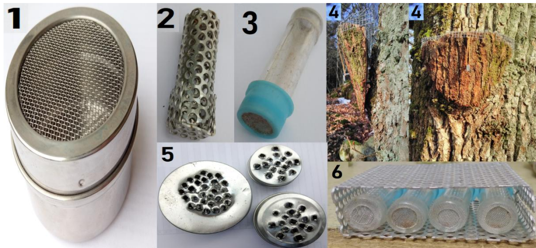
Figure 3 1. Sifter jar with metal net on one side, 2. metallic tube cage with room for one larva, 3. plastic tube with room for one larva, 4. oak cages with room for cassettes (6) containing several plastic tubes and 5. metallic jars in three sizes with room for one larva.
