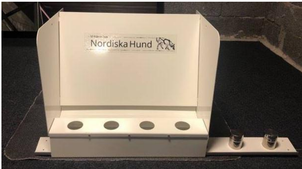
Figure 4 The platform designed to teach dogs to search for specific scents.
