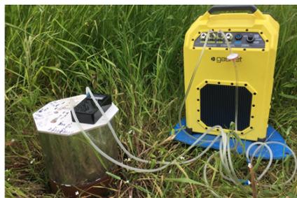
Fig. 2: Left: The field experiment at Brodöbo has a randomized block design with different amounts of sand additions. A represents the control plot (turquoise), B 2.5 cm foundry sand (white) and C 5 cm foundry sand (orange) mixed into 10-15 cm topsoil. Each plot is 8 m by 4 m and is vegetated with timothy (*Phleum pratense*). Right: GHG flux measurement with manual opaque chamber and Gaset GT5000 Terra portable gas analyzer. (Photo: Antonia Hartmann).
