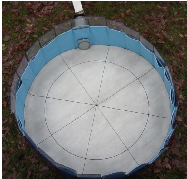
Figure 3: Arena experiment set up consisting of an arena divided into 16 sections and a pipe connected to it with a door at each end.
