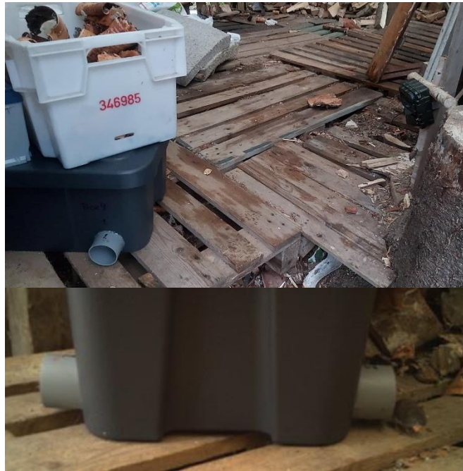
Figure 4: 'Vole box' set up. The top picture shows the camera trap facing a box placed in the human dwelling and the bottom picture shows the tube going through the box where voles can run through.
